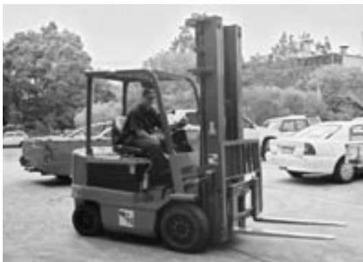
A risk assessment made this business change from diesel to electric powdered forklifts. This helped reduce air pollution and protected personnel.
