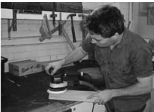
Portable sanders with extraction units fitted to collect particulate and dust emissions produced during the sanding process.
