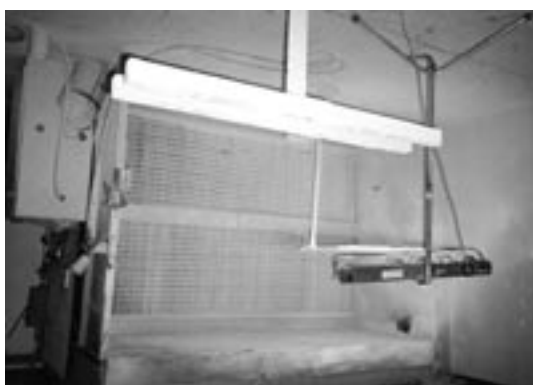
Open faced spray booth with a dry cardboard filter and heat curing lamp used in the finishing process.
