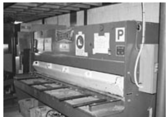
A guillotine used for cutting sheets of metal prior to welding activities are conducted can produce particulate and dust emissions that can be harmful to the health of personnel and the environment.
